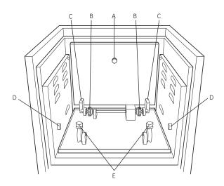
Fig 2. Hybridization oven drive components
